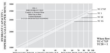
15 20 30 40 50 60 70 80 90 100 PRESSURE DROP ACROSS HYDRANT – POUNDS PER SQUARE INCH Note: Pressure drop change in pressure head from water main at hydrant base to hose.
